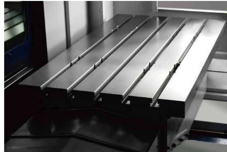
Fine ground table surface with excellent flatness.
